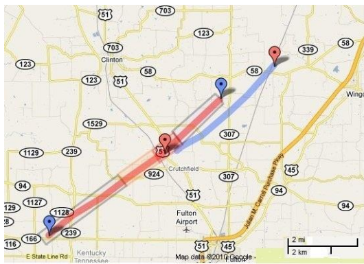
Figure 21. Map of damage survey for the 2 May 2010 event. The red line represents the tornado path while the blue line represents the RFD wind damage path. The boxes around the tornado path are used to depict tornado rating (EF0, EF1, EF2, EF0 from southwest to northeast). Yellow lines are roads labeled with highway numbers. Click image to enlarge.
